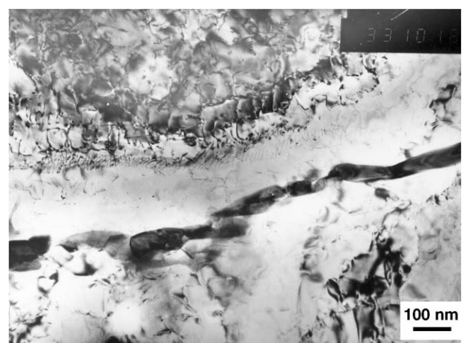
Fig. 13. Precipitates of type \text{M}_{23}\text{X}_6 on a grain boundary in cold-worked ChS-68 steel at 520 °C and 71 dpa.
